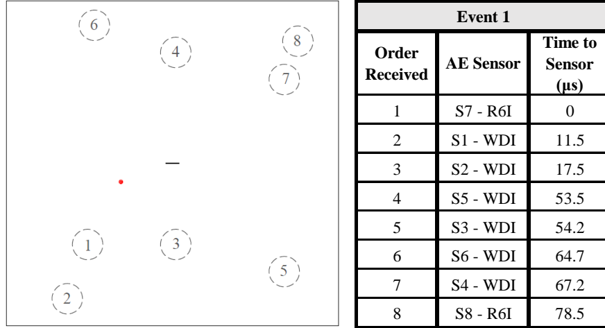
Figure 4.25: Event 1 order of response, corresponding sensor, and time to sensor
