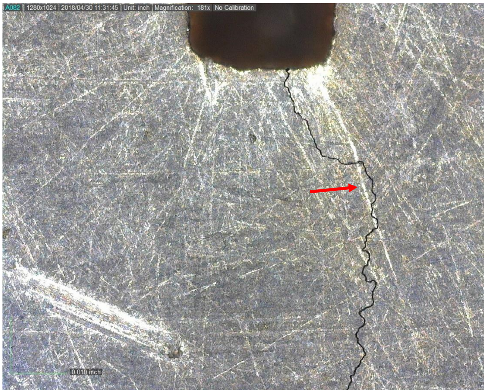
Figure 4.33: Post cracking at notch at day 19
