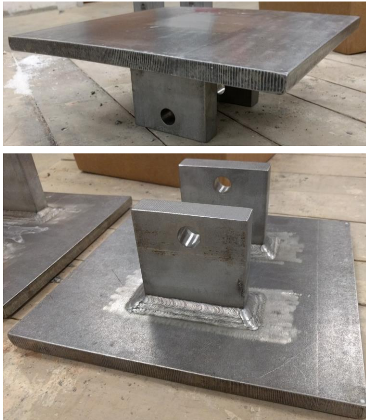
Figure 3.4: 304H stainless-steel specimens with starter notch
