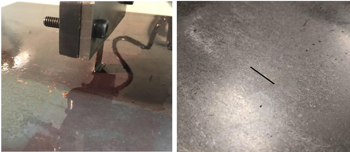
Figure 3.7: Electrical discharge machined notch
