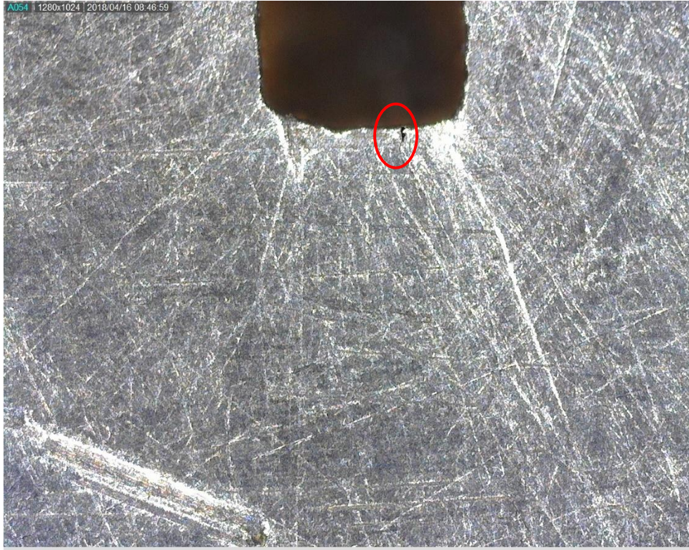
Figure 4.32: Initiation of cracking at notch at day 9 of 19
